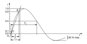
Waveform of short current (8  $\mu\text{s}/\text{20}\ \mu\text{s})$  at the output of pulse generator
